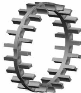
Fig. 4. One-piece finger-type cage.
