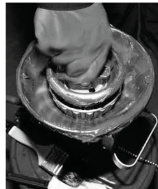
Fig. 15. Mechanical grease packer.
