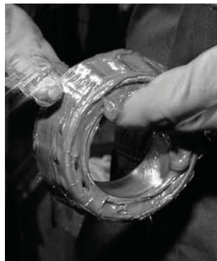
Fig. 14. Grease can easily be packed by hand.
