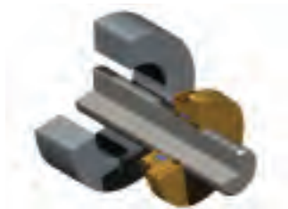
Figure 14: Seal Installation on Shaft
