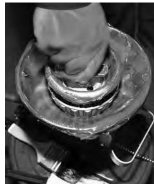
Fig. 11. Mechanical grease packer.
