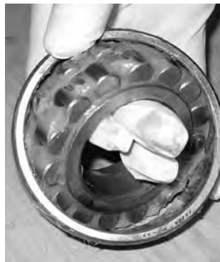
Fig. 10. Grease can easily be packed by hand.
