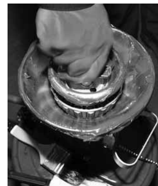
Fig. D-11. Mechanical grease packer.
