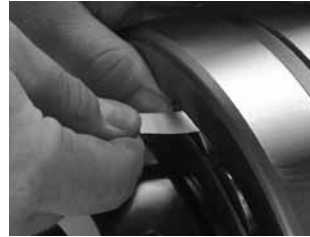
Fig. D-3. Measure RIC before installation.
