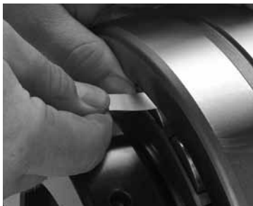
Fig. D-7. Measure RIC before installation.
