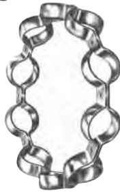
Fig. 52. Pressed-steel welded cage.
