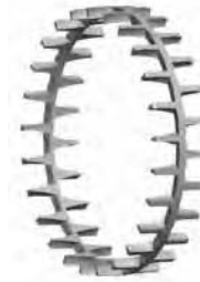
Fig. 45. One-piece, machined-brass, land-riding, finger-type cage.
