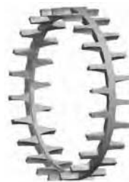
Fig. 44. One-piece, machined-brass, roller-riding, finger-type cage.
