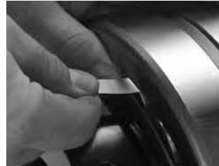
Fig. 91. Measure RIC before installation.
