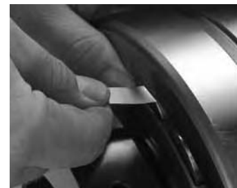
Fig. 95. Measure of RIC before installation.
