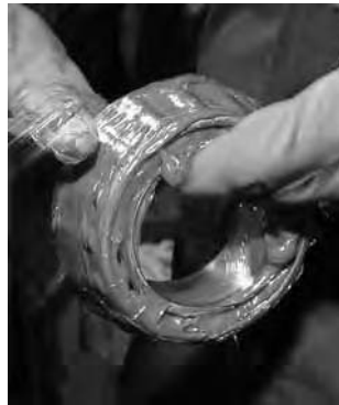
Fig. 147. Grease can easily be packed by hand.
