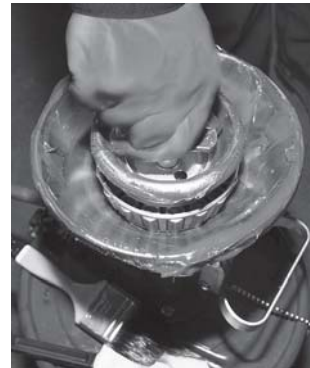
Fig. 24. Mechanical grease packer.
