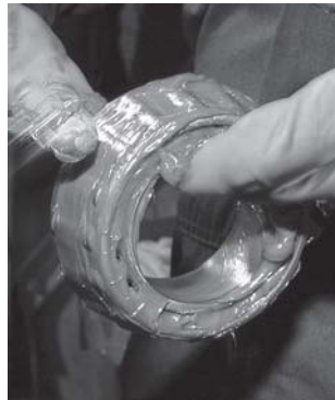
Fig. 23. Grease can easily be packed by hand.
