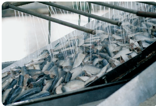
Dacrotized chains used in a fish processing plant
