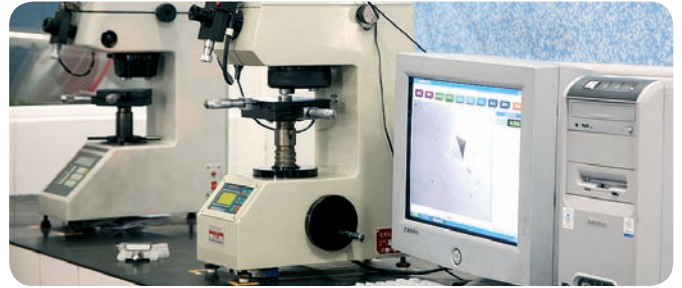
Microhardness testing equipment, where batch tests are done, to ensure hardness is within specification
