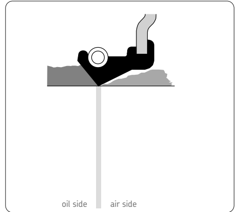
Fig 40. Conventional sealing lip with straight edge
