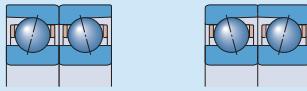
Static axial stiffness for two bearings arranged back-to-back or face-to-face – 72 .. D series
