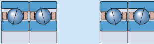
Static axial stiffness for two bearings arranged back-to-back or face-to-face – 718 .. D series
