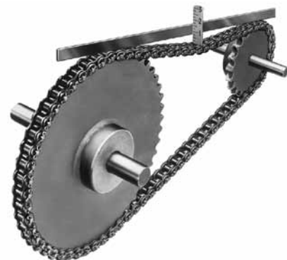
Determining chain sag
