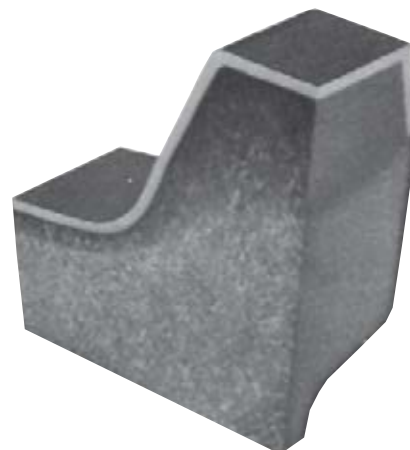
Proprietary induction hardening process gives every heat treated sprocket superior case depths and hardness.
