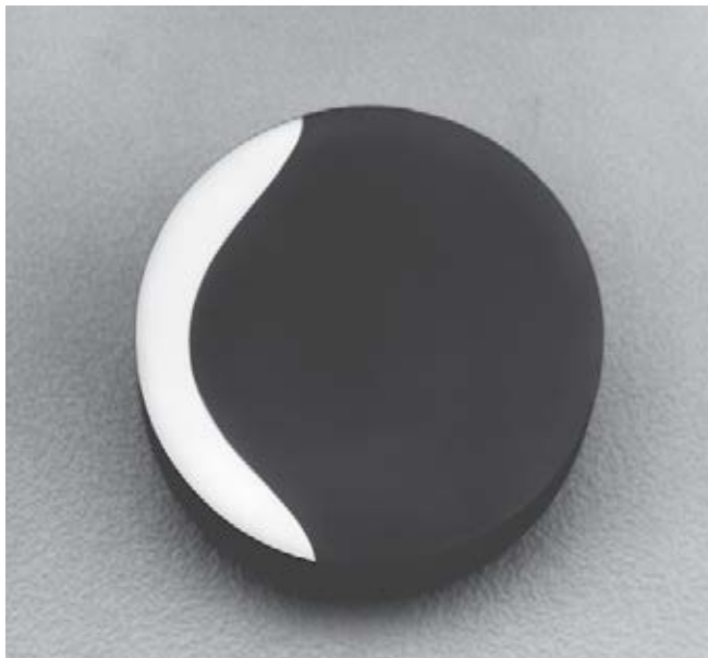
A cross section of a selectively induction hardened WHX pin – the crescent area is super-hardened to dramatically lengthen pin wear life. The balance of the pin material is left in the thru-hardened condition to give the pin excellent toughness.
