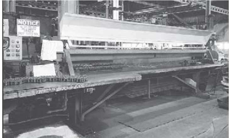
All Cast and Cast Combination chains are 100% inspected and proof tested to ensure that no poorly molded links leave the factory.
