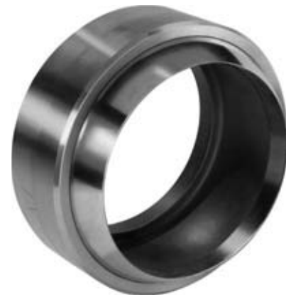
A helicopter swash plate bearing. The PTFE liner in the I.D. of the outer race and the bore of the ball accommodates misalignment and linear motion.
