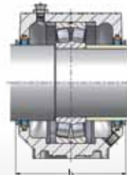
Felt strip seal + V-Ring SC..FS V..A
