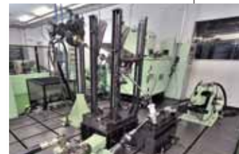
Power Steering System Energy Consumption Measuring Apparatus
