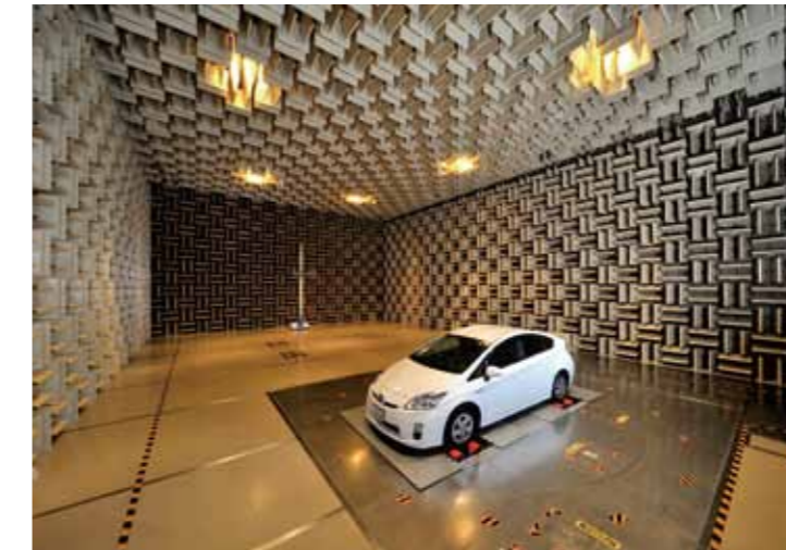
Electromagnetic Anechoic Chamber
