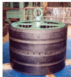
Lifting tool for rolling bearing assembly
