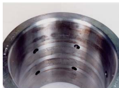
Fretting on bore surface of inner ring
