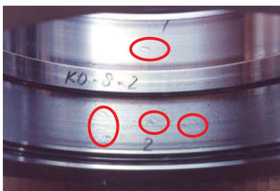
Brinelling on raceway surface of outer ring
