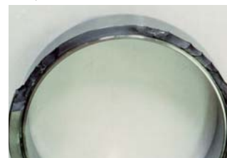
Inner ring cracking
