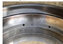
(Outer ring raceway of four-row tapered roller bearing)
