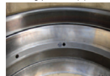
(Outer ring raceway of four-row tapered roller bearing)
