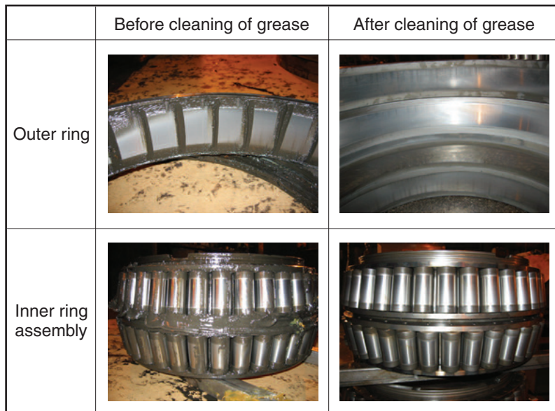
Fig. 5 Post-use appearance of bearing with high-performance seal
