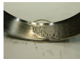
(Outer ring raceway of four-row tapered roller bearing)
