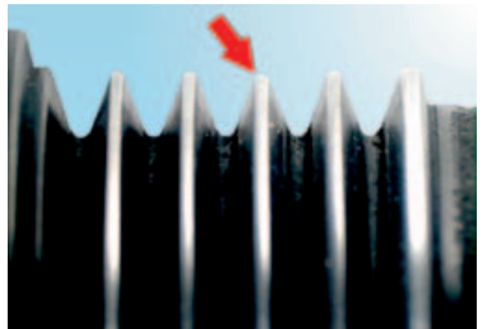
Fig. 3: Worn profile peaks
