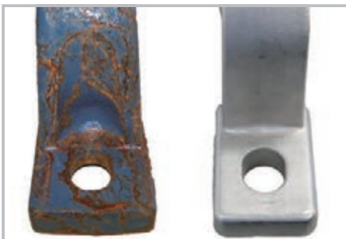
Great performance in demanding salt spray tests (72 hrs) on Stainless units
