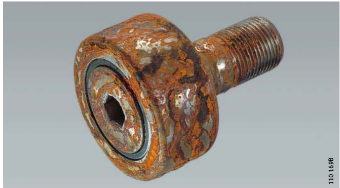
Figure 1 NUKR52 without coating after salt spray test
