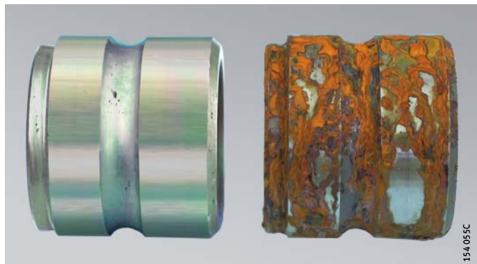
Figure 1 Coated and uncoated part after 24 h in the salt spray test
