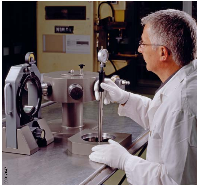
Figure 2 Measuring the raceway diameter of the outer ring
