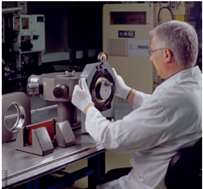
Figure 4 Positioning the enveloping circle gauge
