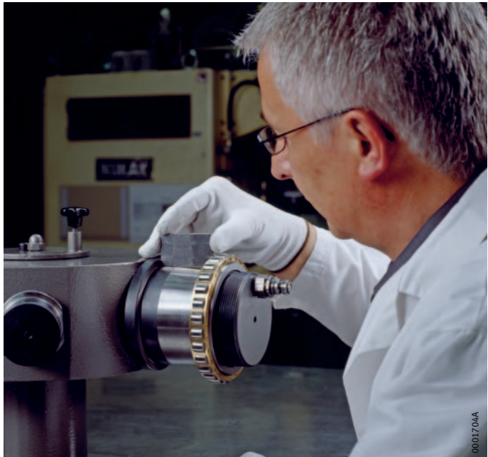
Figure 5 Measuring the distance to the shaft shoulder
