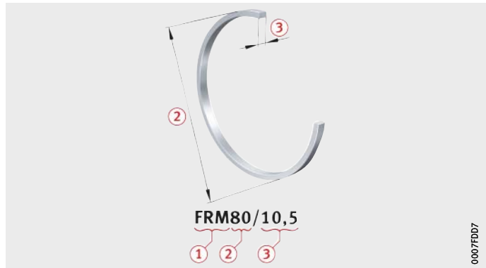
Figure 9 Designation structure of locating rings, example
