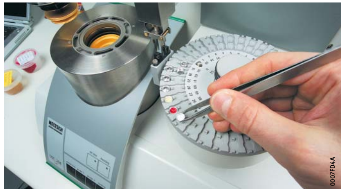
Figure 1 Analysis of the thermal behaviour of greases
