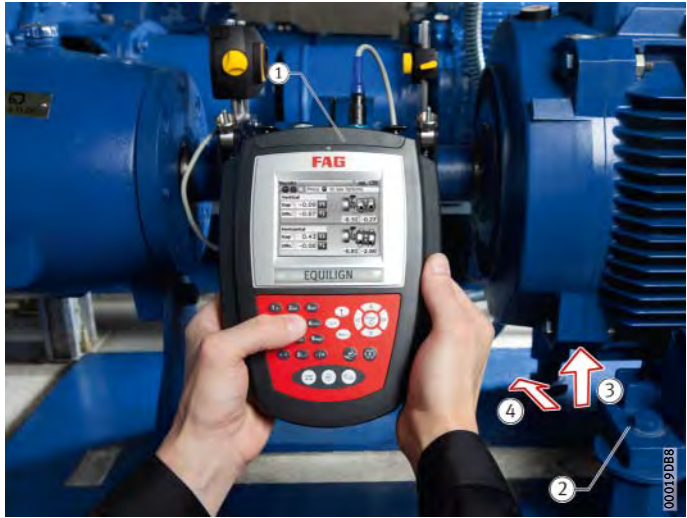
Figure 10 Finding the soft foot
