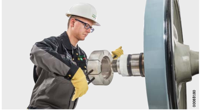
Figure 2 Training on dismounting Inner ring of wheelset bearing
