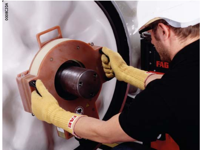
Figure 2 Rigid inductor in the dismounting of labyrinth rings
