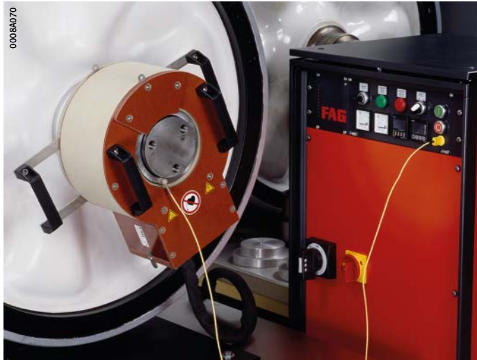
Figure 3 Rigid inductor in the dismantling of wheelset bearings
