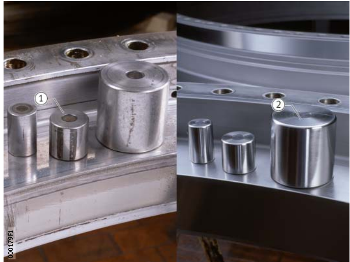
Figure 8 Rolling bearing raceway and rollers before and after reconditioning
